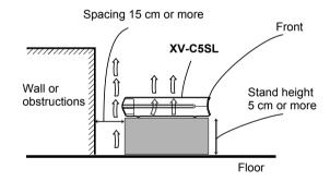
The above illustration shows the case using the horizontal installation. For the other installations, locate the unit conforming to the above illustration and provide sufficient space around the unit.
